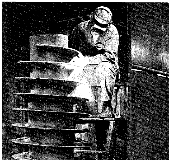
Abrasive materials can be handled economically if the wear problem is systematically analyzed to find the best solution. If abrasion-resistant materials are required, Sharples centrifuges provide an unequalled selection. (See table on opposite page.) Super-D-Canter conveyor flights are shown here being hard-surfaced by one of many special techniques that are employed.
